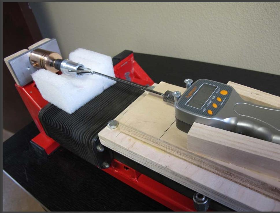
**Force gauge fixture removing a connector**
